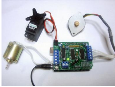
Figure 6.4. Motor Driver Shield is Connected to Stepper Motor, Servo Motor, DC Motor.
