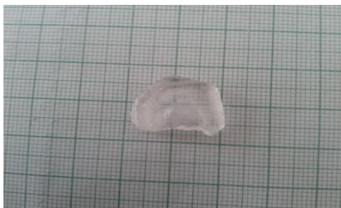
Figure 1. Grown TAC Seed crystal.
