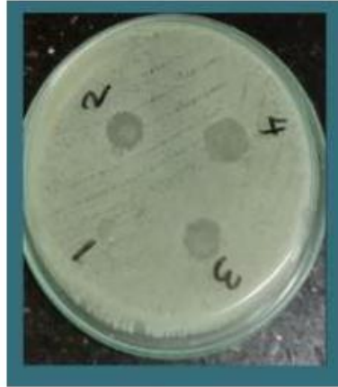
Figure 8. Anti microbial activity of (1&2) cellulose composite against E.coli and S. Aurus (3&4) CMC composite against E. coli and S. Aurus.
