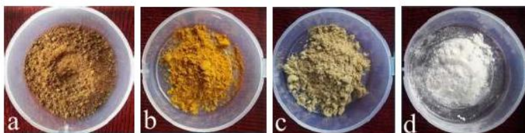
Figure 1 (a). Pure Peanut shell powder (b) alkali treated (c) HNO 3 / ethanol refluxed (d) Micro crystalline cellulose.
