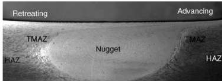
Figure 4. A typical macrograph showing different micro structural zones in FSP 7075Al-T651.
