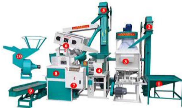
1.Feed hopper 2.Paddy conveyor 3.De-stone machine 4.Rice huller/husking machine 5.Brown rice conveyor 6.Gravity sieve 7.Distribution cabinet 8.Rice polisher 9.Broken rice separator 10.The chaff crusher
