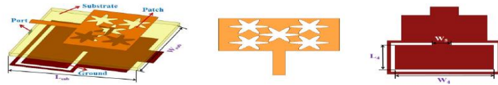
(a) 3D view of proposed antenna (b) DMA (c) SRR inscribed ground
