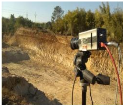
Figure 2. High speed video camera of 1000fps capacity.
