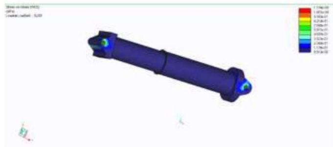
Figure 4(b). Displacement distribution on gas spring.
