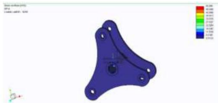
Figure 3(b). Displacement distribution on hub.
