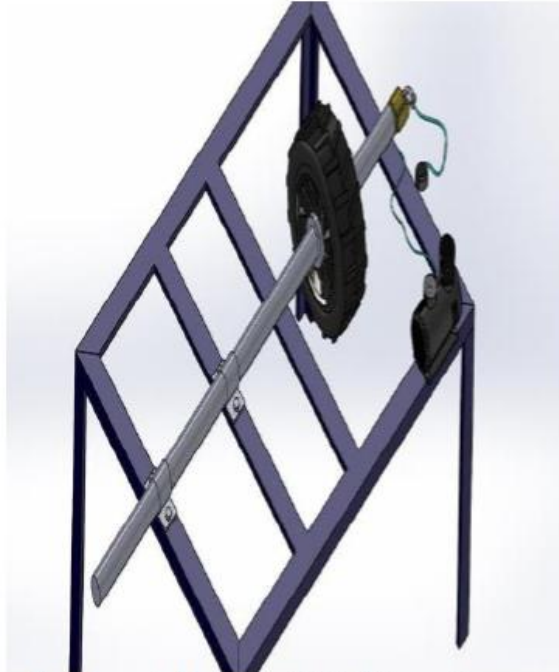
Figure 3. Isometric view of tyre self-inflating tyre system.
