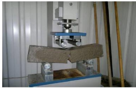
Figure 4.5. Flexural strength test of concrete (Source by Calculation).
