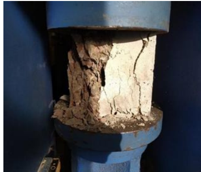
Figure 4.1. Compressive strength of concrete.
