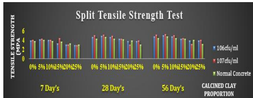
Figure 3. Predicted Split Tensile Strength test result of Bacterial Concrete.
